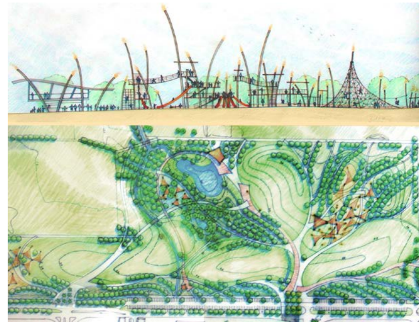
Fig. 174. Early drawing illustrating how the overall 'flowing' design language is applied to both the general layout of the park and the design of specific architectural elements, like the main children's play area
