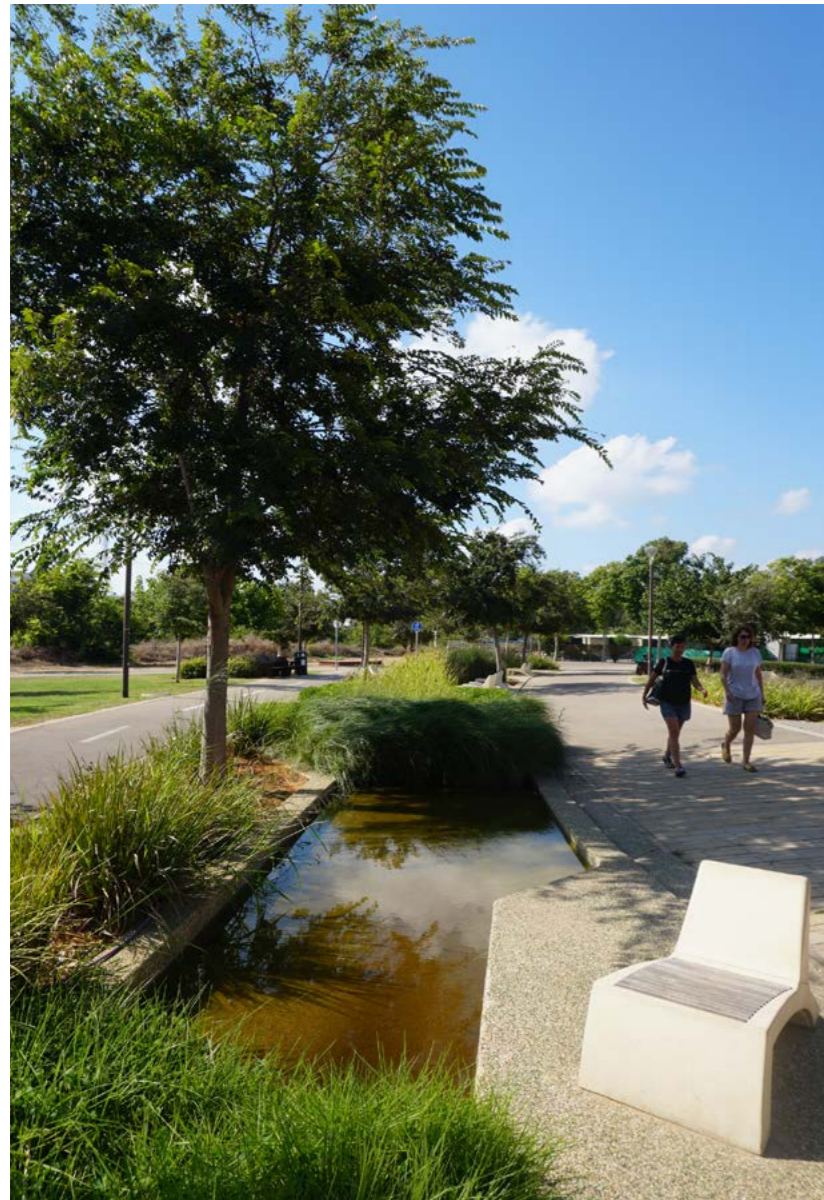
Fig. 232. A water level of no more than 10cm allows for free access and play. Water flows between open areas and planted wetlands which cool and filter the water before being circulated back to the source pool
