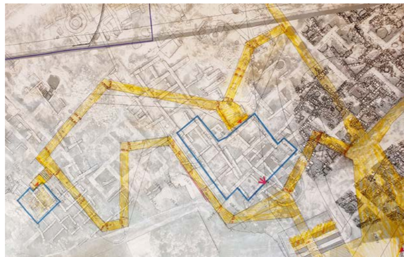
Fig. 139. We designed the layout and heights of the proposed path system located within an archaeological site by studying the combined information from the aerial photograph and the ground survey, Archaeological Park Tel Beit Shemesh, Barbara Aronson, Noga Nevo, 2021
