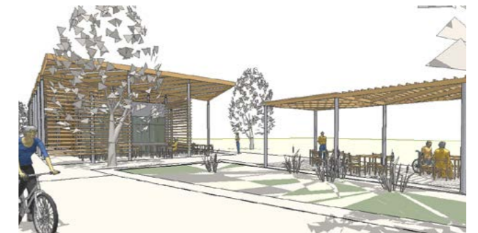
Fig. 234. 3d explorations from different stages of the design. Most construction drawings were generated from the 3d model of the building
